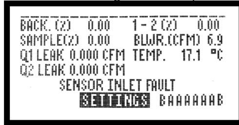
Figure 18. Status message on display with “Sensor Inlet Fault”
