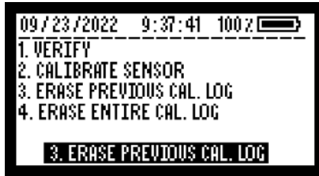
Figure 22. Erase of Previous Calibration Log
