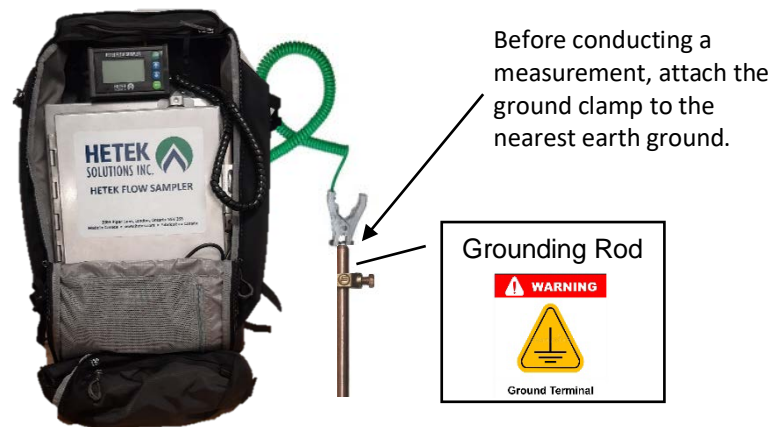
Figure 5. Hetek Flow Sampler with Grounding Clamp and Cable Assembly
