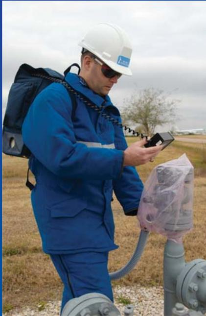
an enclosure measurement. This portable, intrinsically safe, battery-powered instrument will give you the ability to accurately measure leak rates of all natural gas components. This is accomplished by sampling at a large flow rate (between 5 and 10.5 cfm) to completely capture all the gas leaking from the component. By accurately measuring the flow rate of the sampling stream and the natural gas concentration within that stream, the gas leak rate can be calculated.
